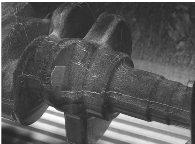
FIG. A1.4 Crankshaft with Various Longitudinal Indications
